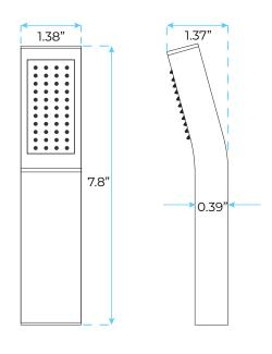
The minimum required water pressure is 0.05 MPa (0.5 bar). Flow rate 2.5 GPM (9.5 LPM).
